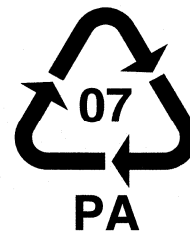
Fig.8 Other plastics. The acronym of the plastic is put under the recycling symbol. In this example: PA = polyamide.
